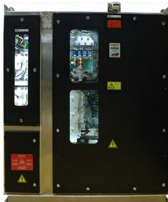
Outside view of Auxiliary converter
