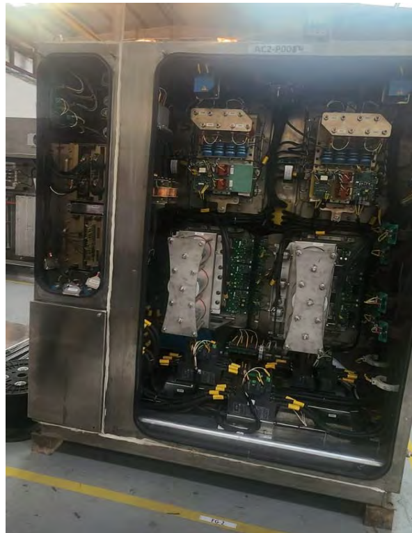
Auxiliary Converter (under assembling process)
