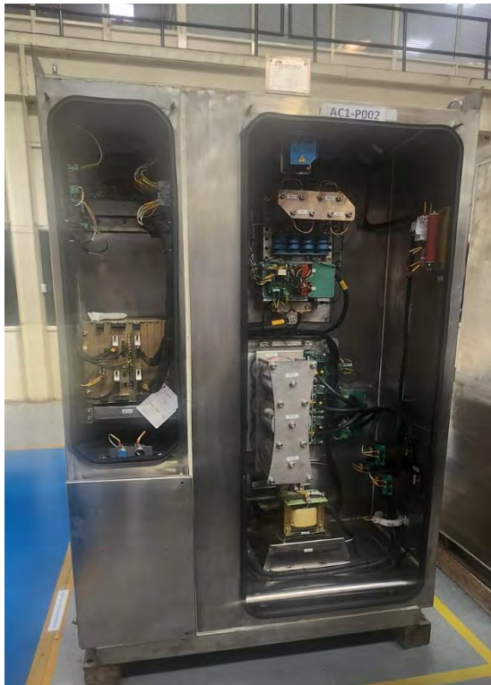
Auxiliary Converter (under assembling process)
